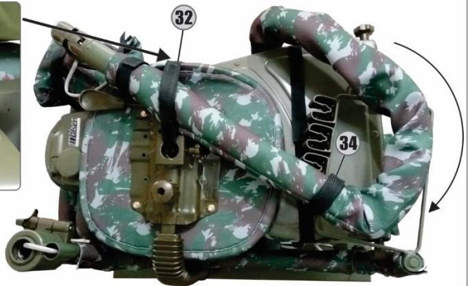
18 - Position the operating light's arm with the headlight on the backrest chair as in the picture above, attach the dental stool seat with the 105 cm strap (32) and pass the strap through the opening in the seat chair frame (33). Attach the tray frame to the operating light's arm with the 40 cm strap (34).
