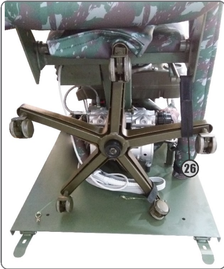
16 - With the 40 cm strap secure the dental stool base on the seat adjustment lever (26) and make sure that the hoses and the electric cable will not be loose.
