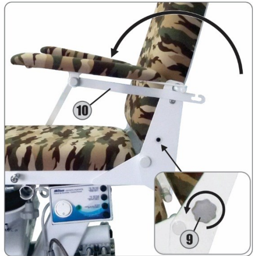
9 - Remove the handle from the left side of the backrest (9), position the metal rod (10) in parallel with the armrest and rotate the armrest counterclockwise and remove it; repeat the operation with the right armrest.
