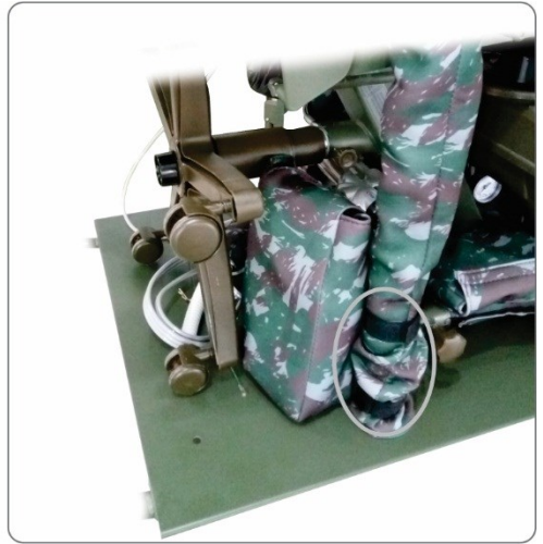
20 - Attach with Velcro® strap the packaging of water tanks on the operating light's arm.
