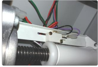
To remove the plastic cover under the seat, find and remove the 5 plastic rivets from the plastic cover. You will reach the motor for seat inclination. Disconnect the black cable from the limit switch, press the seat inclination command for 5s in order to have more seat elevation. Remove the plastic cover and connect the black cable again on the same connector.
