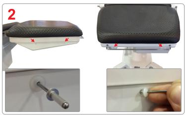
Find the 6 plastic rivets which hold the legrest plastic cover and remove them. Push the center pin (of plastic rivet) by using a metal rivet or a 1mm Hex screw. After pull it out.
