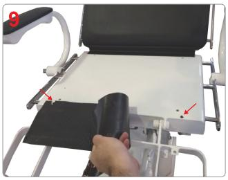
Remove this piece of PVC coat, and carefully remove remaining material from metal frame.
