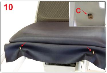
Place new seat upsholtery and put the 4 brass philips screws only using hands (C). After place all screws, tighten them. Place the screws for legrest at the metal frame passing through the PVC coat holes.
