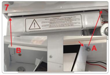
To remove the battery set, lose the screw (A) but don't remove it. Remove the battery set from its fitting.
